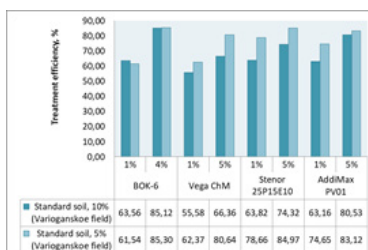
Figure 1. The enhanced washing efficiency for standard sandy soil contaminated with 5 and 10 wt% of light crude oil (0.84 g/cm 3 )
