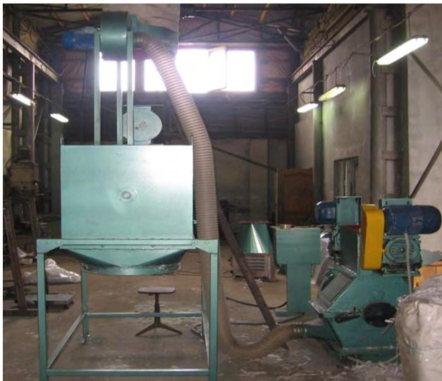
Fig.1. Photo of universal crusher separation type DS-150 "IMEX", for separation of polymer-containing waste paper (wallpaper, packaging) to obtain two fractions: 1- loose cellulose-ecowool, as a heat-insulating material for insulation of residential premises in construction, and 2 - fractions of crushed polymers of PE, PVC ..
