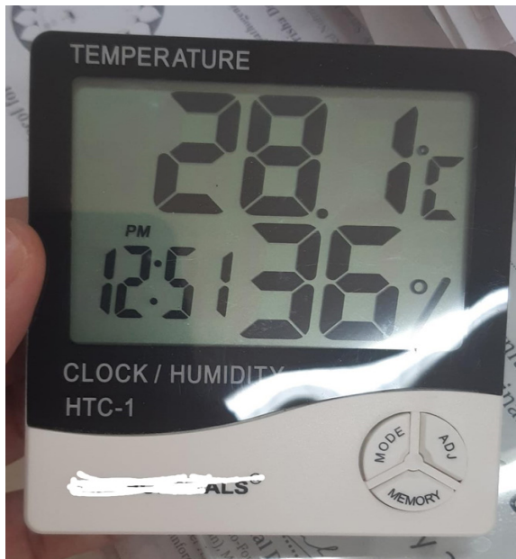
Figure 2) Digital hygrometer showing ambient temperature, time and relative humidity (anticlockwise from top).
